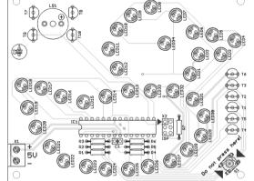
6. LEDs (LED1~LED34): The orientation is important for the LEDs. Make sure the flat side of the LED (cathode) matches the silkscreen outline. The flat side of the LED also corresponds to the shorter lead. Start with 3 or 4 LEDs, one in each corner, then add the other LEDs one at a time. Try to avoid bending the leads outward, as this will make it harder to remove the LED again. Don't solder too long on the LEDs, they will have reduced brightness if they become too hot during soldering.
