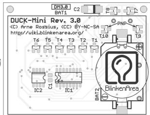
**5. Resistor (bottom):** Solder the resistor (marked "2701") between IC2 pins 5 and 7, as shown to the right. Make sure the contacts and solder don't touch pin 6. (A bridge between pins 7 and 8 doesn't matter.)
