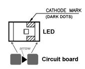
1. LEDs (top): The orientation is important for the LEDs. You can see two small green (or dark) dots inside the LED on one side (cathode). This side must face in the direction the little arrow on the board is pointing to, as shown above. All LEDs face the same way. Don't solder too long on the LEDs, they will have reduced brightness if they become too hot during soldering. The kit contains a spare LED in case you break one.
